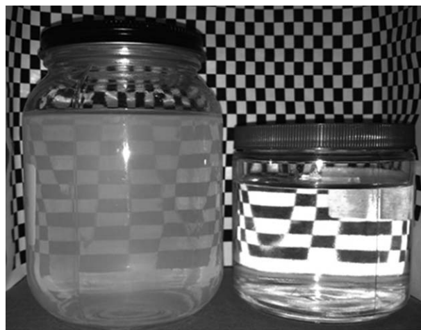
Figure 6. Improperly water-reduced CUPs (left); properly water-reduced CUPs (right).
